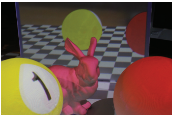
Figure 6: An example of hybrid rendering. Notice the correct occlusion of spheres and physical bunny and the missing reflection of the bunny in the mirror.
